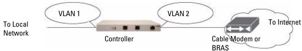
Figure 2 IP Address Assignment to VLAN via DHCP or PPPoE
